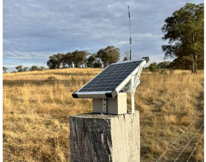
Fig. 1. Solar-powered remote node mounted to fence post.
