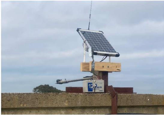
Fig. 5. Remote node with water level sensor deployed on a water storage tank.
